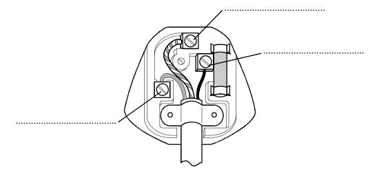
(b) (i) Explain how the earth wire and the fuse protect a person from an electric shock when there is a short circuit to the metal case of an appliance.
