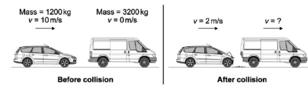
Use the information in the diagram to calculate the velocity, *v*, in metres per second, with which the van moves forward after the collision.
