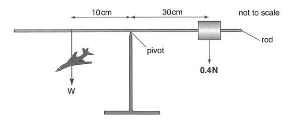
The rod is balanced horizontally on a pivot by a 0.4 N weight.
