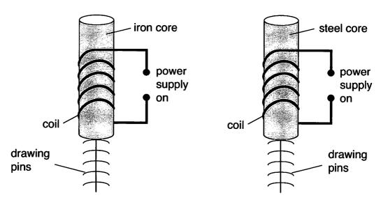
The diagram shows the greatest number of drawing pins which each electromagnet could hold when using the same current.
