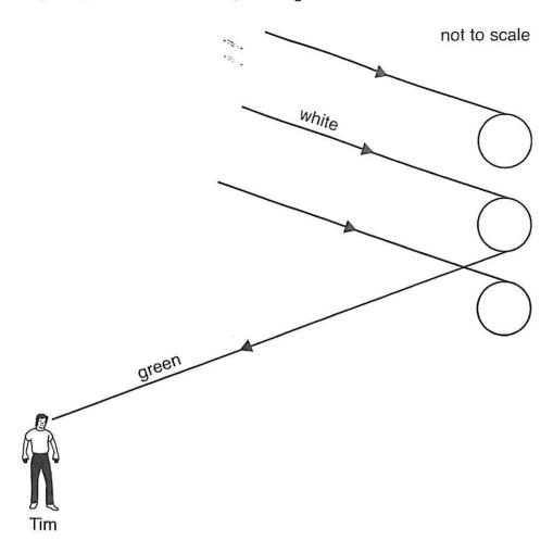
The light reaching Tim has reflected off the back surface of the raindrop.
