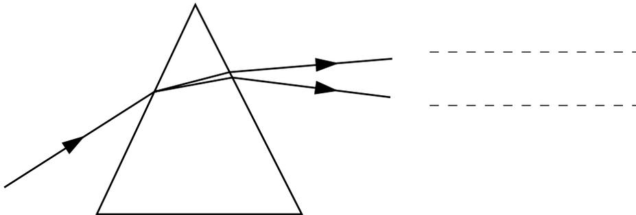
The prism splits the light into several colours. The two extreme ends are shown. Write beside each of these rays which colour it **could** be. (3)
